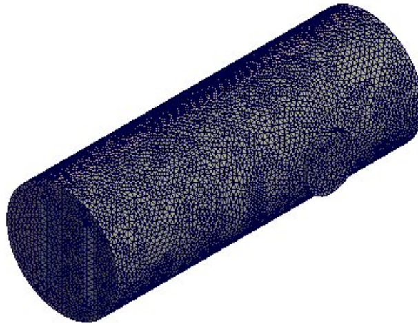
Fig. 4: CFD Mesh of Air Porous Model (545,591 elements)
