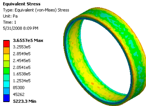
Fig. 10: Thermal Stress Distribution in the Tube
